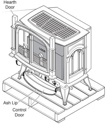
Figure 7 - Opening Control Door and Removing Hearth Door
